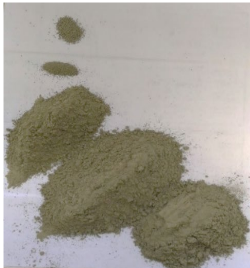
Fig. 2. Sieved Portland Limestone Cement
