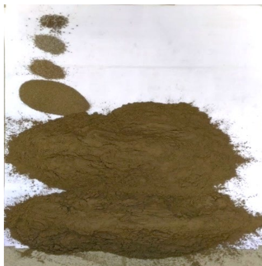
Fig. 3. Sieved Spent Bleaching Earth Pozzolan
