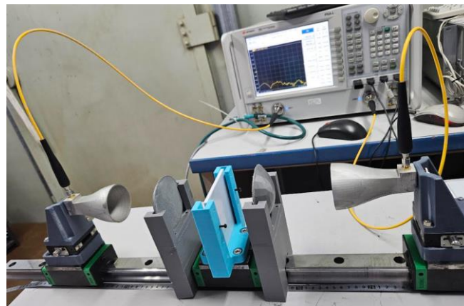
Fig. 12. Measurement setup with lens for 3-D printed horns
