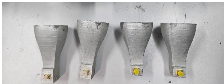
Fig. 10. 3-D printed horn antennas
