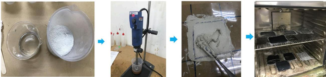
**Fig. 1.** Glass fiber reinforced geopolymer composites (GFRGCs) fabrication process
