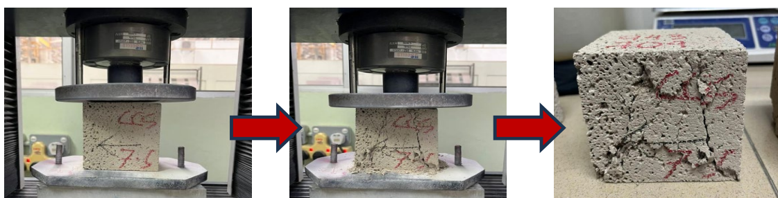
Fig. 3. Compressive strength test
