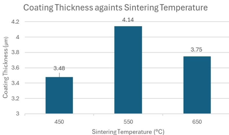
**Fig. 4.** Effect of sintering temperature on the coating layer thickness
