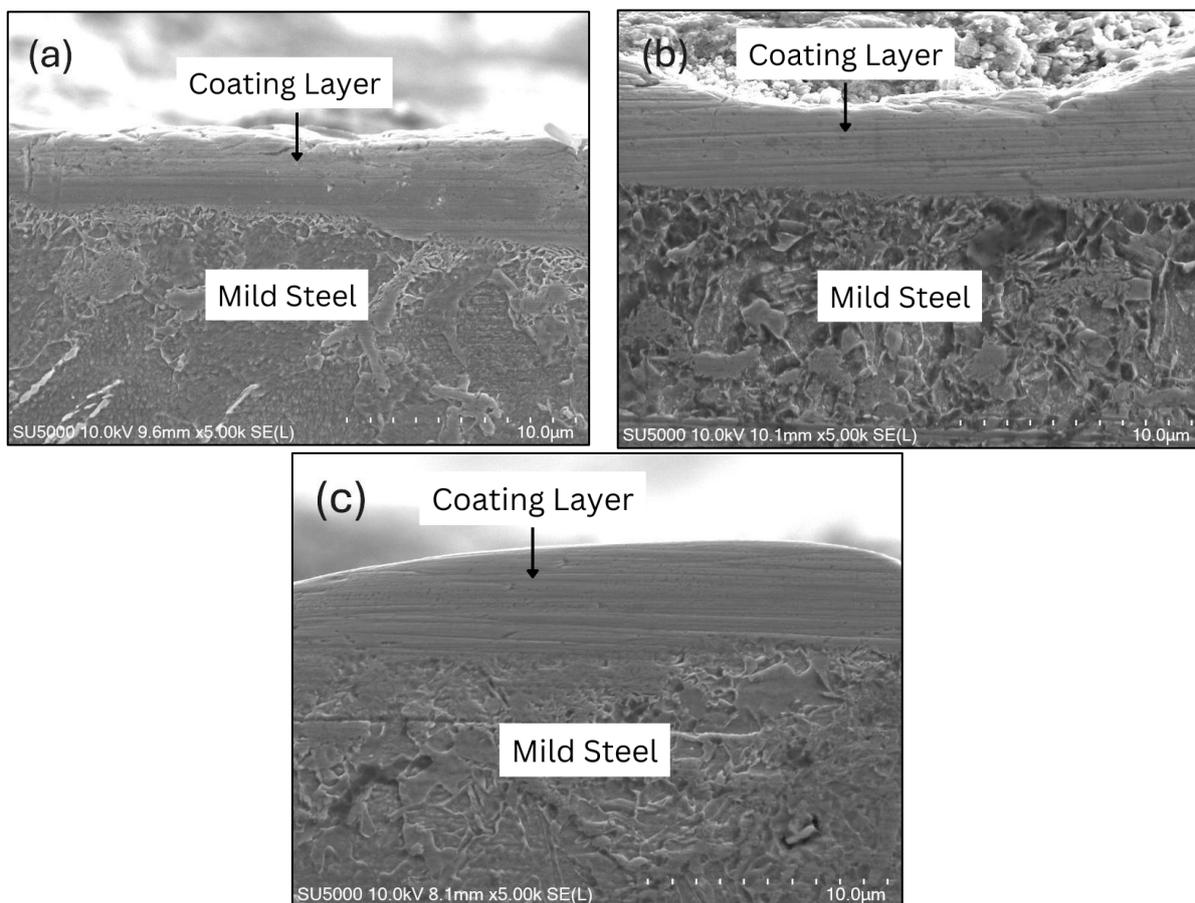
**Fig. 5.** FESEM of coating layer thickness under different sintering temperatures (a) 450 °C, (b) 550 °C, and (c) 650 °C
