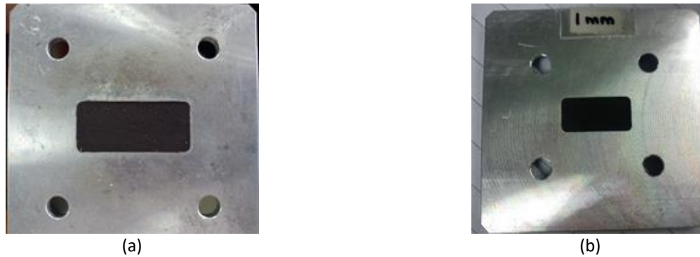
Fig. 2. Sample holder at (a) X-band and (b) Ku band
