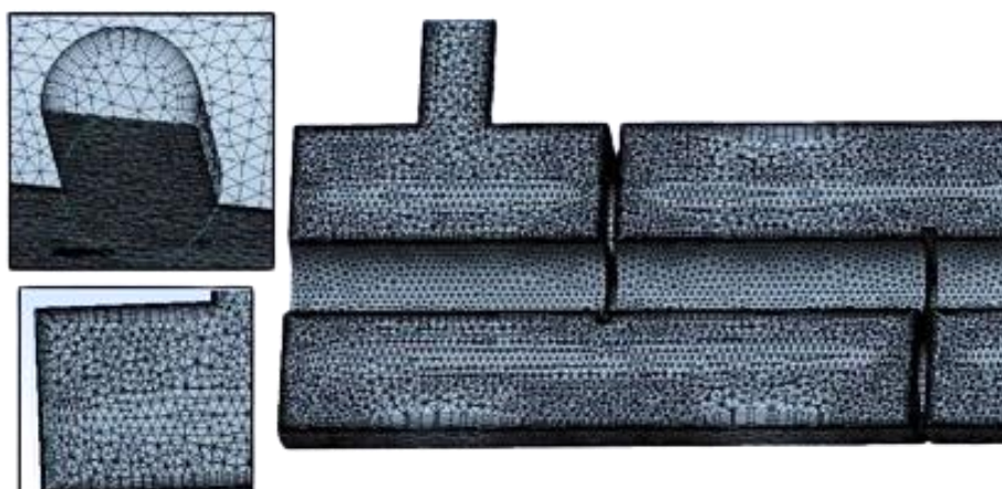
Fig. 7. Initial inflation layers
